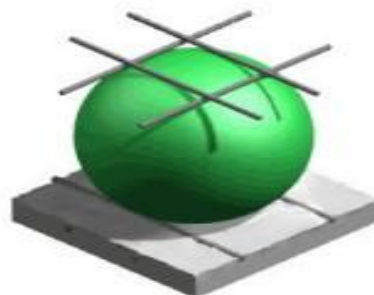
Fig.1.Reinforcement mesh over HDPE balls
